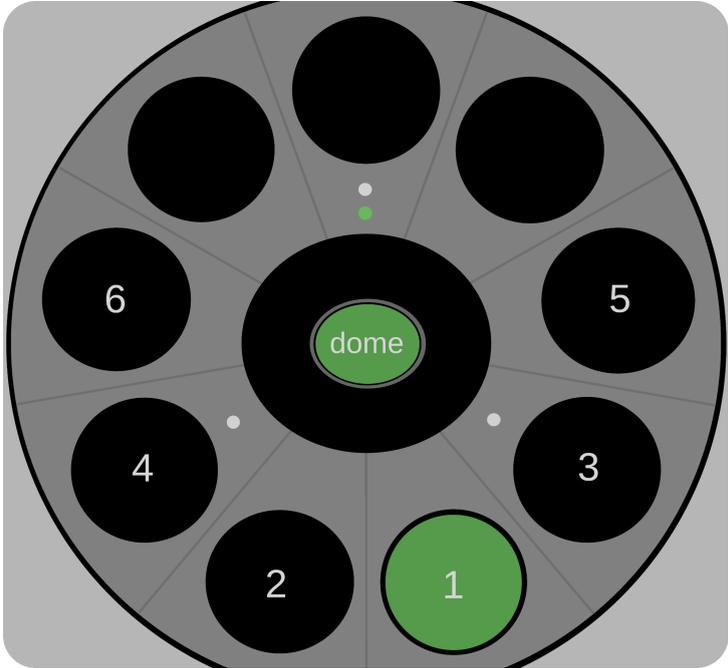
You can switch between instrument scales by holding down the DOME and one of the side tonefields simultaneously for 2 seconds. You can choose 6 scales by default:
