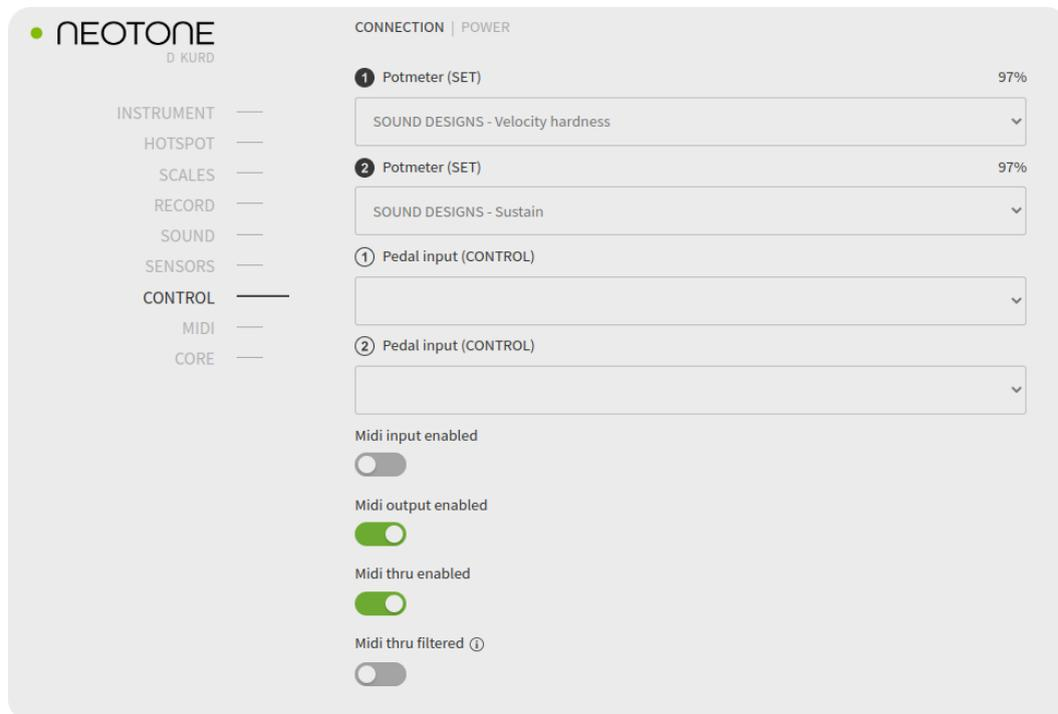
Most of the sliders and switches can be paired up with a back panel knob or foot pedal. This function allows you to change any settings on the interface by physically making adjustments on the instrument (no WiFi connection needed). For example, if you have paired up KNOB 1 with the volume slider, even when the instrument is not connected to WiFi, you can adjust the volume by physically turning KNOB 1.
