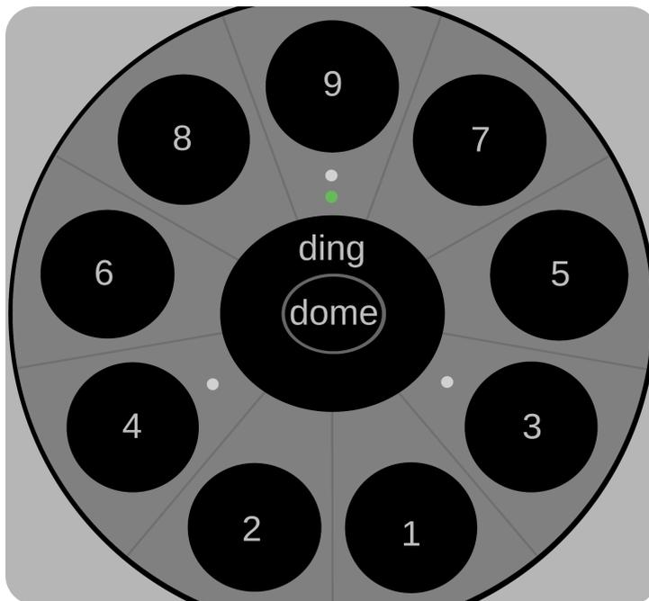
There are 4 inlay markers on the body of the instrument, for orientation. The double marker points to the highest note. The two other markers point to note #3 and #4. It's easy to find the highest note as the double marker has an indicator light built in.
